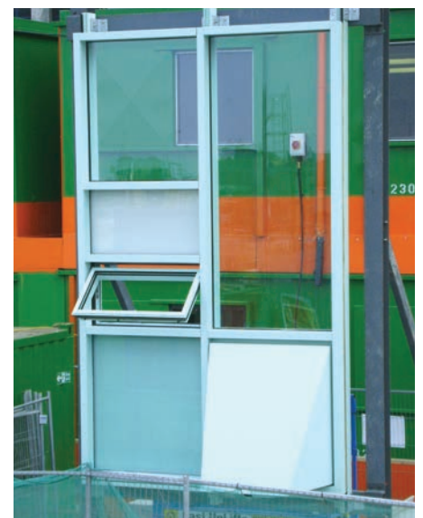
Full-scale cladding mock-up
